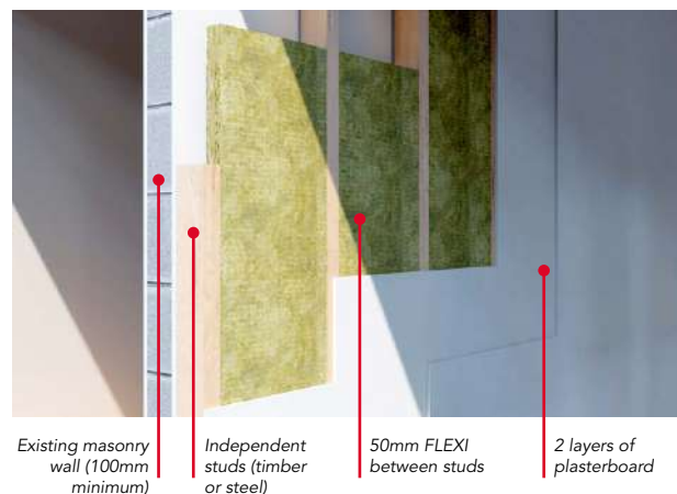
Figure 12 Acoustic applications – separating walls
